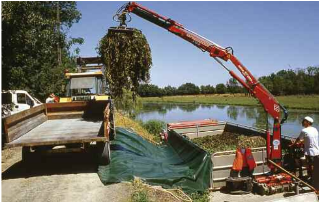
A claw used in the Marais Poitevin marshes to transfer water primrose from a barge to a trailer.
