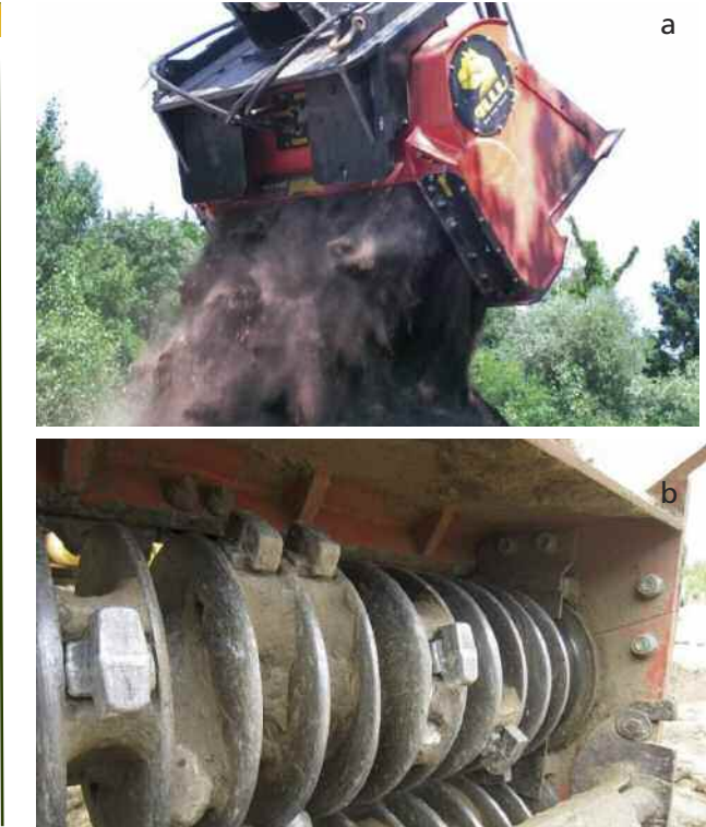
Mechanised management of knotweed in the Gard department, a) soil grinding, b) grinding rotor in the bucket.
