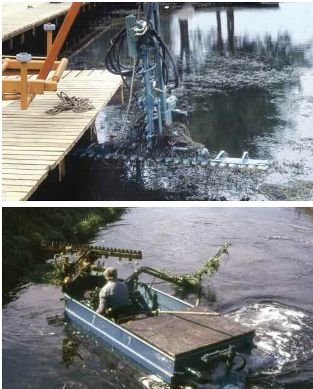
Mowing boats equipped with cutting bars in front and on the side.
